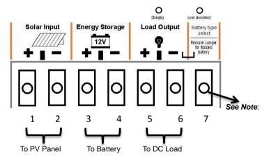
The first pair of screw terminals is the input terminal for solar panel connection. The second pair of screw terminals is the bi-directional terminal used for battery connection. This acts as an output terminal for battery charging from the PV panel through the unit and acts as an input terminal for battery discharging to DC load through the controller.
