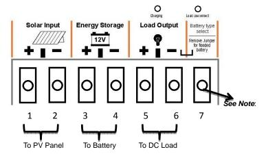
The first pair of screw terminals is the input terminal for solar panel connection. The second pair of screw terminals is the bi-directional terminal used for battery connection. This acts as an output terminal for battery charging from the PV panel through the unit and acts as an input terminal for battery discharging to
